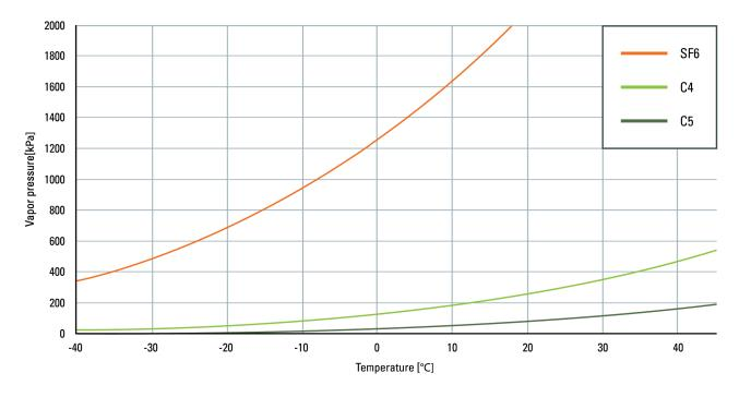
Figure 1: Vapour pressure curves of pure  $SF_{6}$ , C4 and C5 in the temperature range from -40 °C to 45 °C. This curve describes the pressure at which a substance liquefies dependent on the temperature. In the area below the curve, the substance is gaseous, above the curve it is liquefied.
