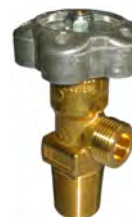
Valve for new SF 6 gas *, reconditioned SF 6 gas as well as used SF 6 gas with a SO 2 content of < 250 ppm v in accordance with DIN 477 no. 6 W21.8 x 1/14"Brass
